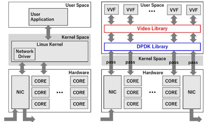
Figure 2. High-speed VVF using DPDK (right) and Normal DPDK usage (left)
