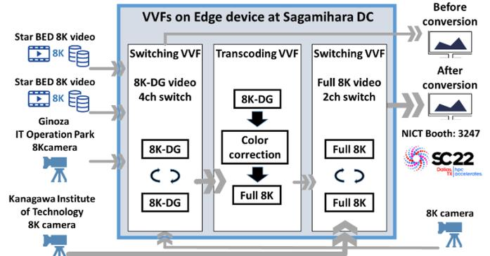
**Figure 5. Uncompressed 8K UHD video workflow by chaining multiple VVFs**
