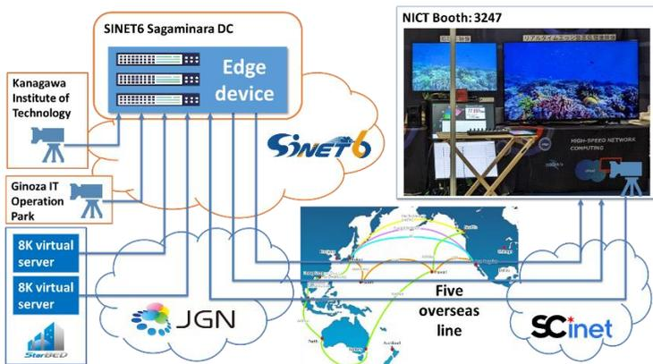
**Figure 7. Network topology and traffic flow of the demonstration**
