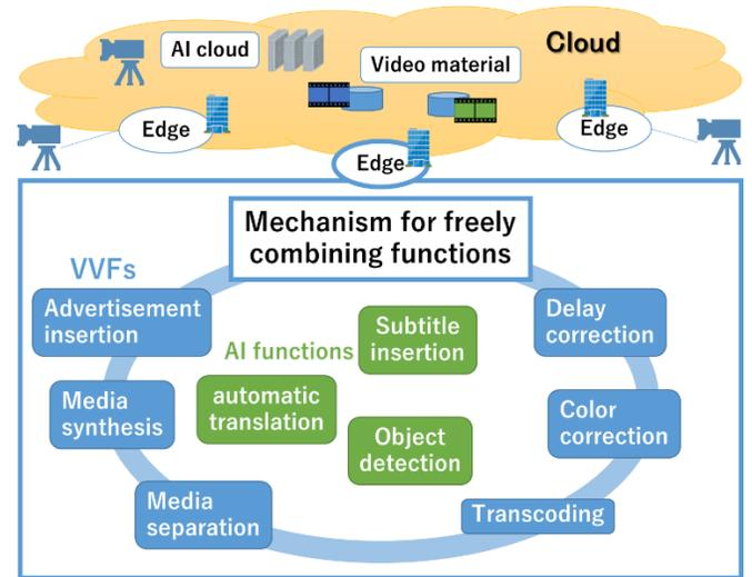
Figure 1. Cloud-based UHD video processing platform
