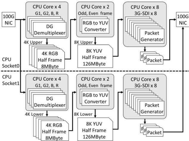
**Figure 3. Implementation of transcode function**
