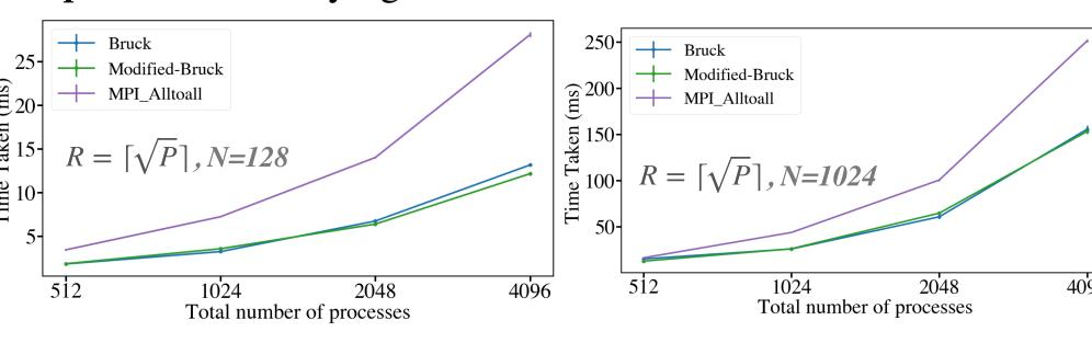
The Bruck algorithm with r near  $\lceil \sqrt{P} \rceil$  works well in most cases.
