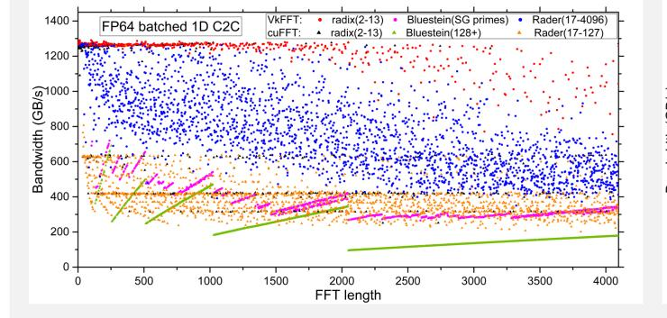
For double precision, both VkFFT and cuFFT use radix decomposition for sequences representable as a multiplication of arbitrary number of primes up to 13.
