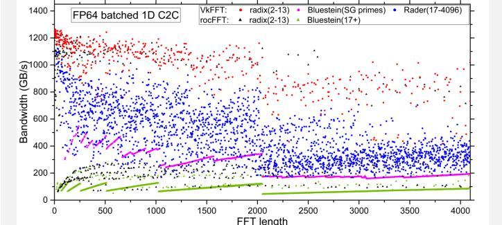
For double precision, VkFFT uses similar to A100 configuration: radix decomposition for primes up to 13, Rader FFT algorithm for non-Sophie Germain primes up to 4096, Bluestein's algorithm for other sequences.
