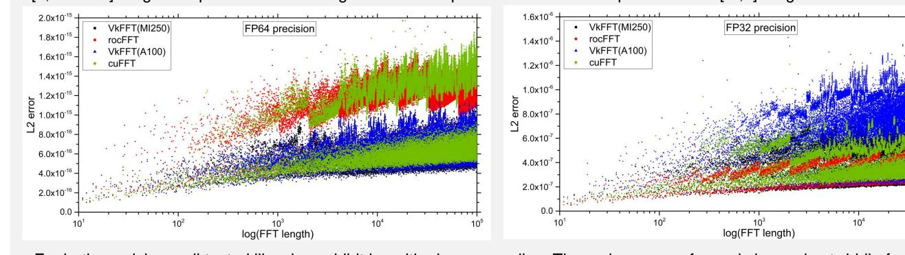
For both precisions, all tested libraries exhibit logarithmic error scaling. The main source of error is imprecise twiddle factor computation – sines and cosines used by FFT algorithms. For FP64 they are calculated on the CPU either in FP128 or in FP64 and stored in the lookup tables. With FP128 precomputation (left) VkFFT is more precise than cuFFT and rocFFT.
