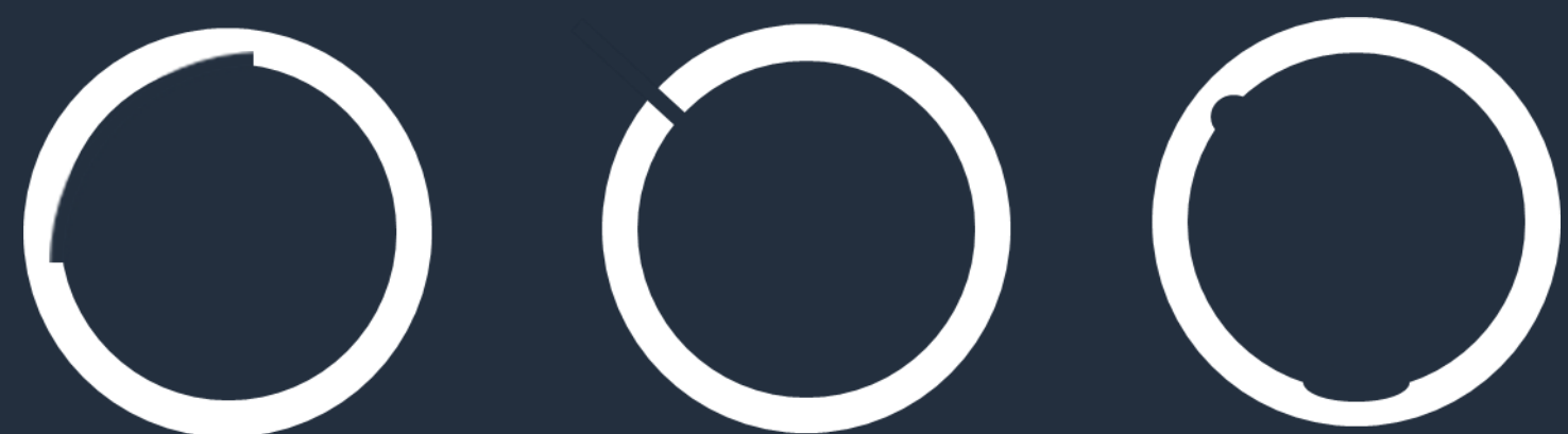
Metal losses may affect a large, shallow area (left), while others penetrate casings (middle). Yet others may be present in multiple regions (right)
