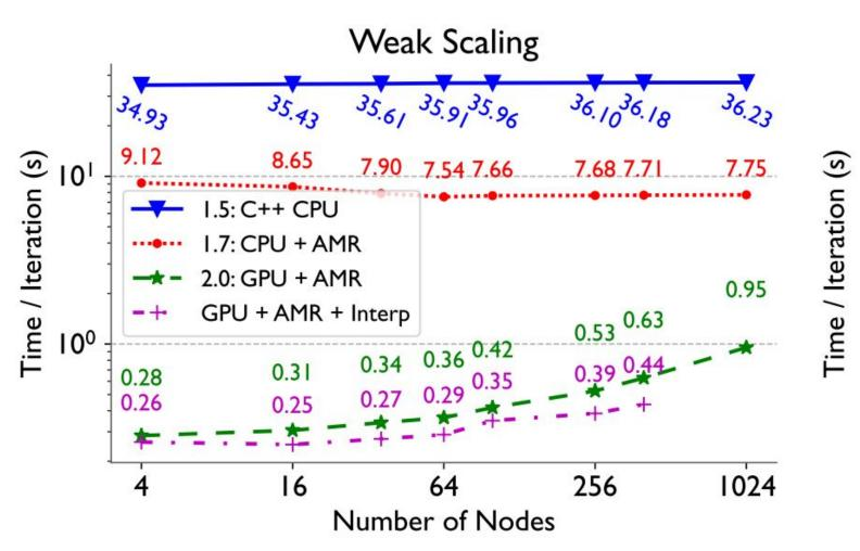
We ran strong/weak scaling of curvilinear DMR on OLCF Summit [4] for GPU runs (NVIDIA V100, 6 per node) and LLNL Quartz [5] for CPU (Intel Xeon E5, 36 cores/node).
