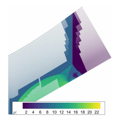
Validated and benchmarked with double mach reflection (DMR) problem, which has been extensively studied [3], using all curvilinear code features.
