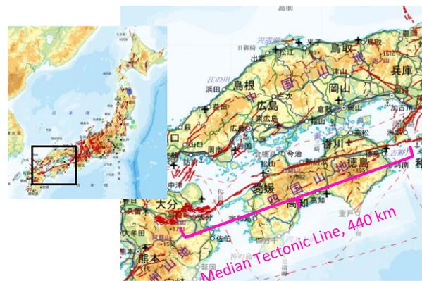
Fig. 1. Geometries and distributions of inland active faults (red lines) on the Japanese Island. Median Tectonic Line active fault is the largest one among more than 100 major faults.
