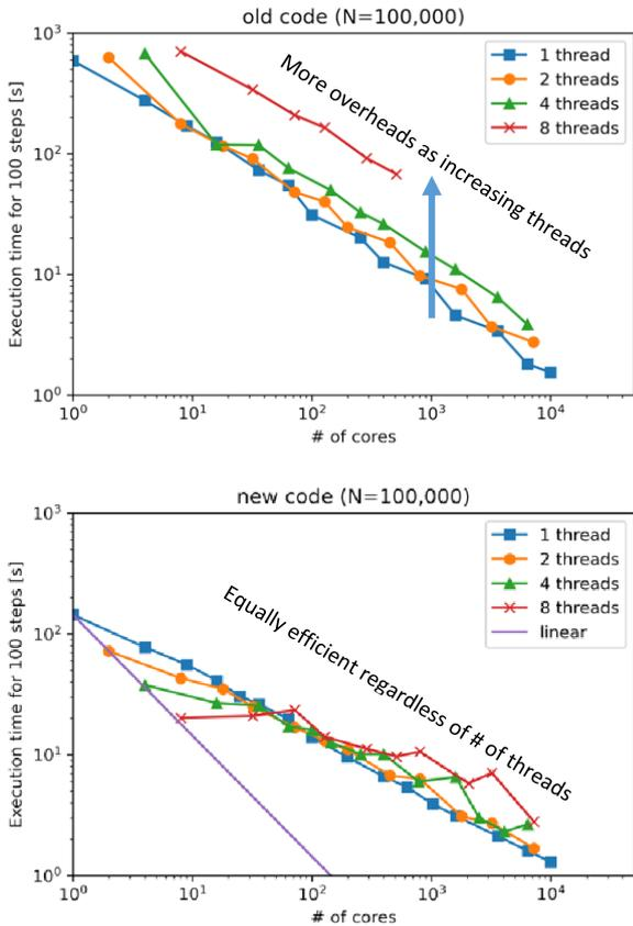
Fig. 2. Scalability of the optimized algorithm. Strong scaling evaluation of the code without optimization (top) and that with the contiguous memory placement (bottom)
